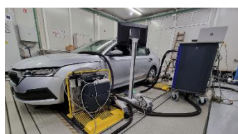
Figure 4: Chassis dynamometer facilities at Laboratory of Applied Thermodynamics
